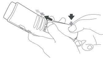
**3** Slide battery cover back over the compartment with pressure on both top and bottom of the battery cover.
